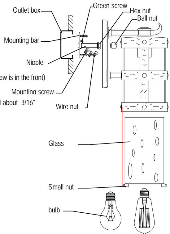
4. Fasten the white fixture lead to the white wire in the outlet box. Fasten the wires together with an approved fastener (wire nut). Starting about 1" below the fastener, tightly wrap the connection with electrical tape so that the connection seals the end of the fastener.
