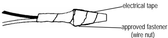
5. Connect the black fixture lead to the black wire in the outlet box. Fasten the joined wires as in step 4
