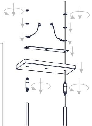
\* Make sure two swivels opening are in the same direction while assembling.
