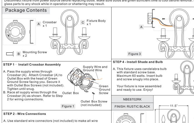
connections. (Connectors are not included with fixture.) Twist connectors until wires are tightly joined together. Wrap each connection with approved electrical tape and carefully stuff all the connected wires into the Outlet Box.
