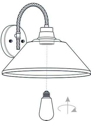
Install the correct bulb referring to fixture markings and/or labels for maximum wattage.
