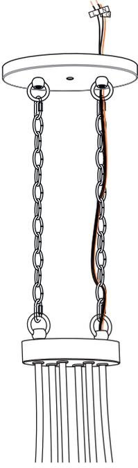
Pull the supply wires with ground wire through the chain alternate links.
