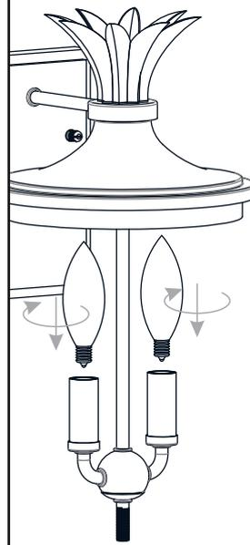
Install two correct bulbs referring to fixture markings and/or labels for maximum wattage.
