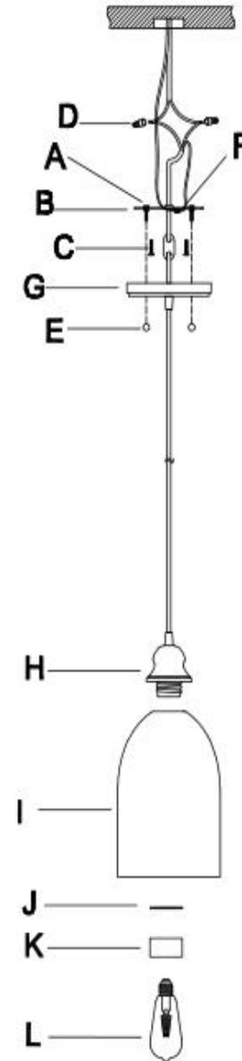
4. Install bulb(K). Be sure to use light bulb(s) with wattage no greater than fixture. Always make sure that electrical current is turned off before char
