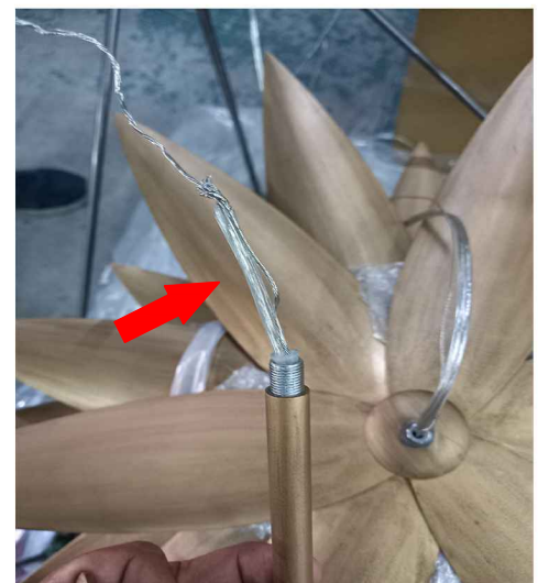
9. SLIP WIRE OVER THE STEM
