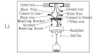
Step.1: Remove mounting bracket (A) from fixture (C) and install to electrical box using screws provided (B). Wire fixture to wires in outlet box. Copper wire is for Ground.
