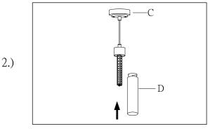
Step.2: Adjust the wire length to desired mounting height. Turn the glass (D) onto cup to secure.
