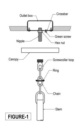
4. Open the end links of the chain and attach the chain to the screwcollar loop. Hang the fixture on the chain at the desired height. Remove the excess chain close all links. Unscrew the threaded ring from the screwcollar loop. Allow the ring and canopy to slide down the chain to the top of the fixture.
